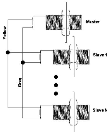
Figure 24 - SYNC Wiring
