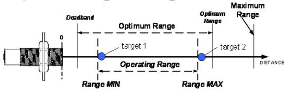
The sensor measures the distance to targets within the *Operating Range* (target 1 to target 2). This range can be set in SenixVIEW by adjusting the *Range MIN* and *Range MAX* parameters. The factory default is the widest possible, *deadband* to *maximum range* (see specifications, page 7).
