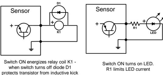
Figure 15 - Sourcing Switch Output Wiring
