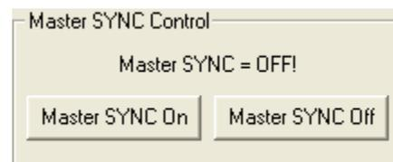
If a Master is detected, click “Master SYNC off” then confirm the status as “No Active Master!” to enable the **Group Control** features. When finished, click “Master SYNC On” to restore SYNC operation.
