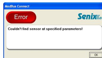
check the (a) wiring, (b) power and (c) interface selections. Check **All Ports** and use **Find Sensor** to scan all sensor addresses at each of 12 ports. Change the port range by clicking **Edit >User Preferences...** and changing Starting Com Port to a higher value. SenixVIEW will identify the first Sensor Model found with the chosen network address on a port. The default is address is 1.
