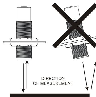
Figure 4 - Sensor Orientation
