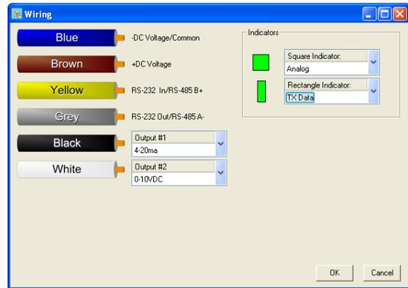
For TSPC-15S, TSPC-21S, and TSPC-25P sensors the following 9-wire dialog appears. Note that each output has a separate wire in these models.
