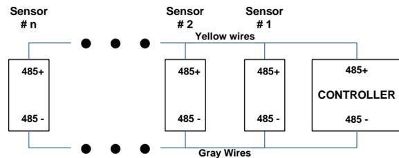
Figure 21 - RS-485 Network Wiring
